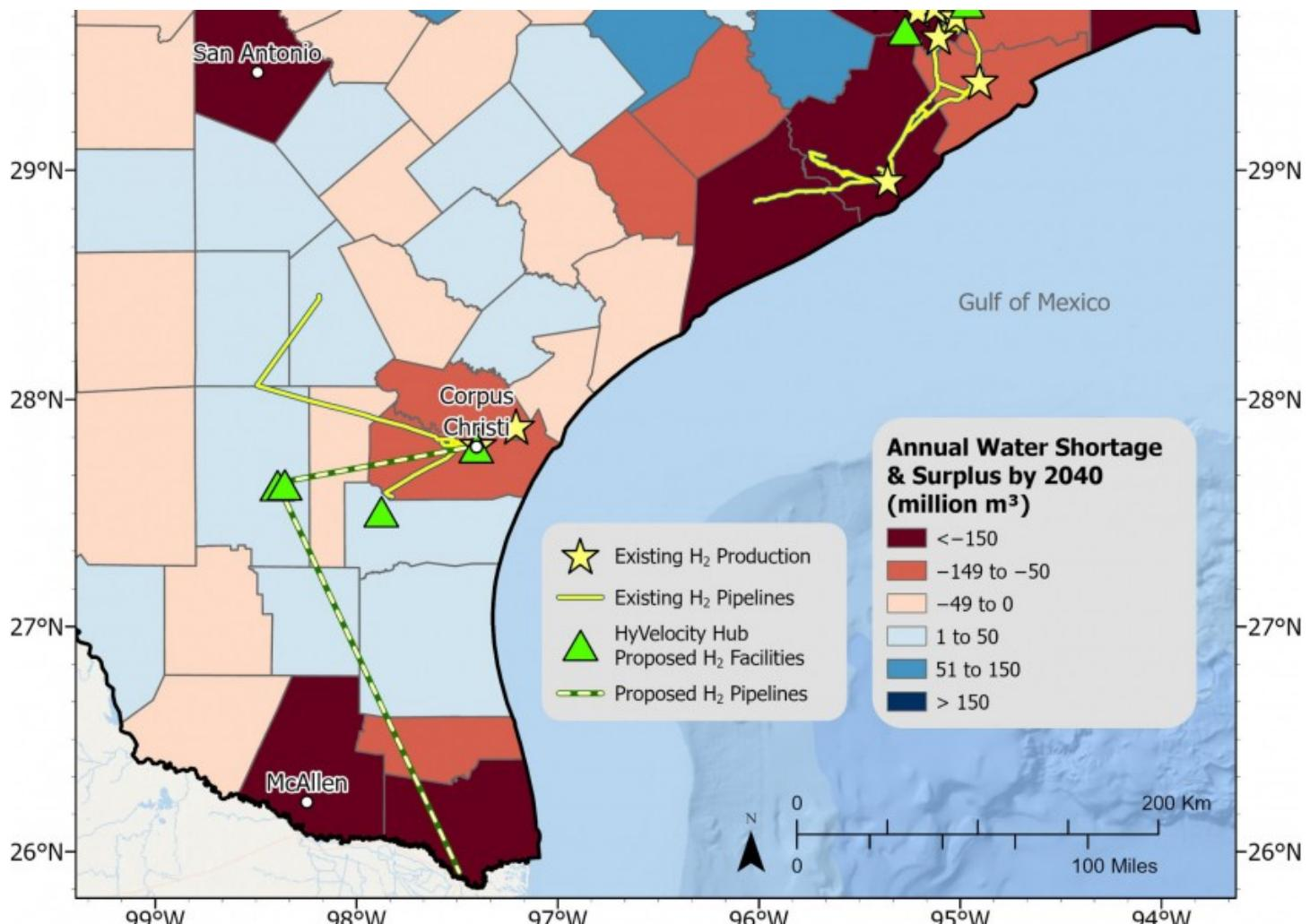
Existing and proposed hydrogen infrastructure as of 2024 in the Gulf Coast region of Texas overlaying projected water needs in each 2040. Credit: Lin et al.
